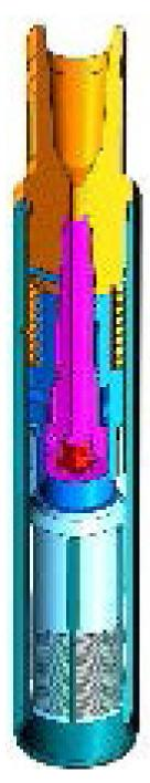
This is a downhole tool used in well intervention for fishing operations. The overshot has a replaceable collet to catch a smooth surface. The collets covers a range of fish outer diameters from 1.0" to 2-1/8"
