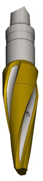
this is a downhole tool for well intervention jobs. Using a mill, it is possible to grind and wash out any object from the well if the hardness of this object is less than the hardness of the mill's cutter. Such an item can be either equipment intentionally run into the well, for example, a bridge-plug, or emergency lost equipment. Rotation of the mill performed by a downhole motor.
