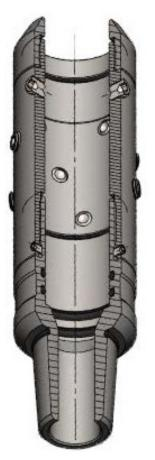
It is the connecting link between the smooth lower end of the CT and any other downhole tool that needs to be connected to the CT for well intervention job.
