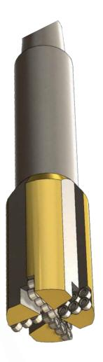
this is a downhole tool for well intervention jobs. Using a mill, it is possible to grind and wash out any object from the well if the hardness of this object is less than the hardness of the mill's cutter. Such an item can be either equipment intentionally run into the well, for example, a bridge-plug, or emergency lost equipment Rotation of the mill performed by a downhole motor.
