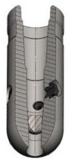
The sand jet perforator can be made in basic design, when the nozzles are open for circulation all the time, or ball activated, when the nozzles are opened only after the ball is droped, which allows you to pressure test BHA or work with tools below the perforator in the BHA.
