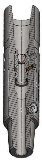
is a downhole tool, run in the hole as part of the borehole assembly (BHA) during the Coil Tubing operations. Normally installed just below the hydraulic disconnect. A certain size steel ball need to be dropped inside the CT from the surface to perform an activation.
