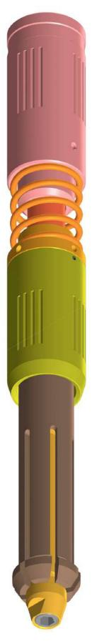
A Flow release spear for a GS profile is a downhole tool that is used to fish and extract from the well Hydraulic Disconnect (HDI) of Marlin Oil Tools' design. When the spear nose enters the pipe, the GS collet securely fixed in the HDI bottom sub, so that it is possible to apply a pulling force to the spear to extract it together with a fish.
